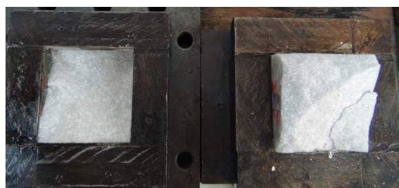
图3 先拉后剪条件下的破裂面 Fig.3 Fractured surface under the condition of tension before shear
