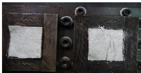
图4 先剪后拉条件下的破裂面 Fig.4 Fractured surface under the condition of shear before tension
